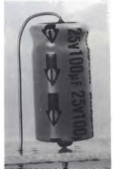
Figure 6: This is an example of an axial lead capacitor mounted in the upright position. When mounting electrolytic capacitors special care must be taken to ensure correct polarity.
